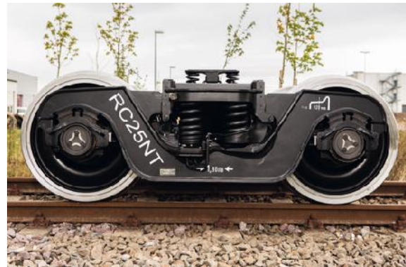
Wheel and track friendly, low-noise and low-maintenance: the RC25NT bogie is designed for heavy-duty freight cars
